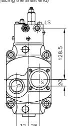
Coding **SU** Spline shaft SAE-C . 14T-12/24 DP
