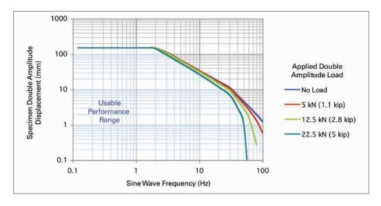
ACTUATOR STATIC FORCE: 25 kN (5.5 kip) ACTUATOR DYNAMIC STROKE: 150 mm (6 in)
