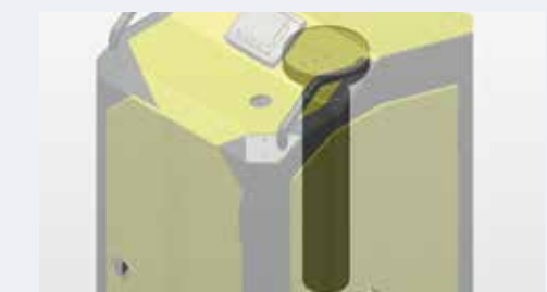
Fig3. Once heated to an optimum 70°C the oil enters a distillation column designed with a dedicated dispersal element.
