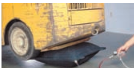
The non-skid space age reinforced inflatable jack is perfect for many applications.
